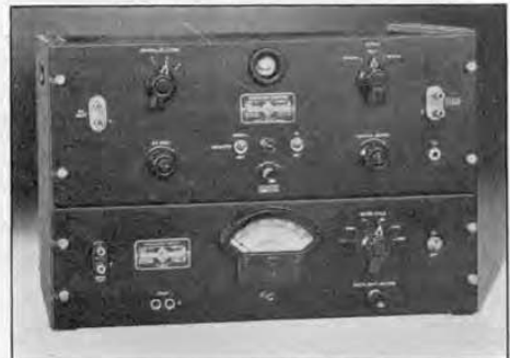
Figure 5. View of a Type 1175-B Frequency Monitor and a Type 1176-A Frequency Meter assembled in end frames.
